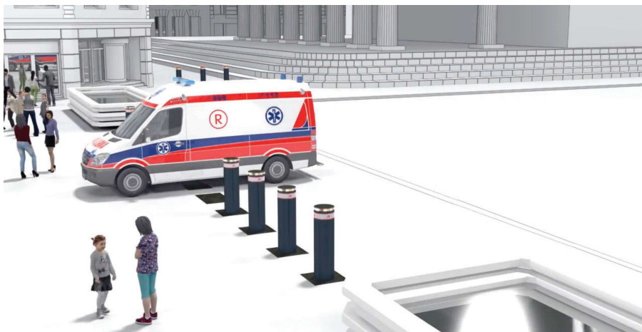
Retractable bollards allow access for emergency vehicles
